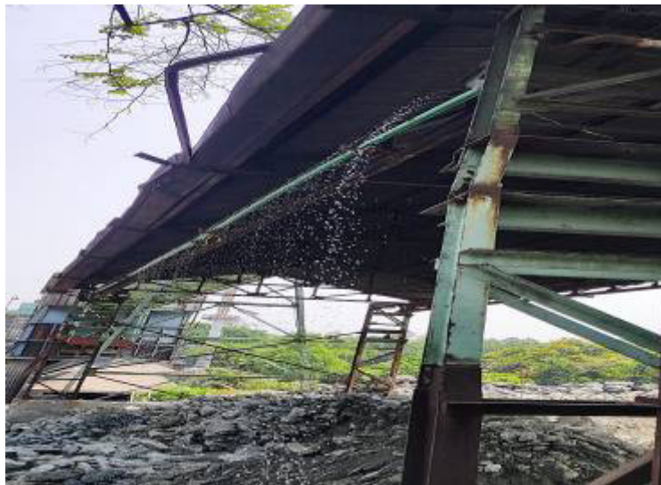
Photographs showing conditioning of the ore with water at the unloading of the ore
