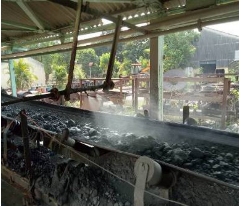
Photographs showing conditioning of the ore with water at the unloading of the ore
